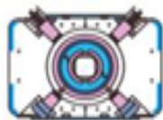
TEVATRON B = 4.5 T Bore : 76 mm
