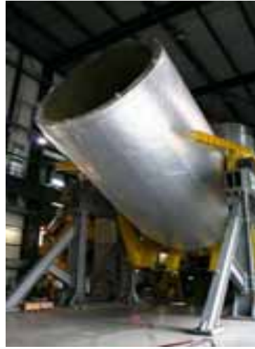
Coil Cooled to 4.5K in 25 days (Feb). Test on Surface (May-Aug 06)
